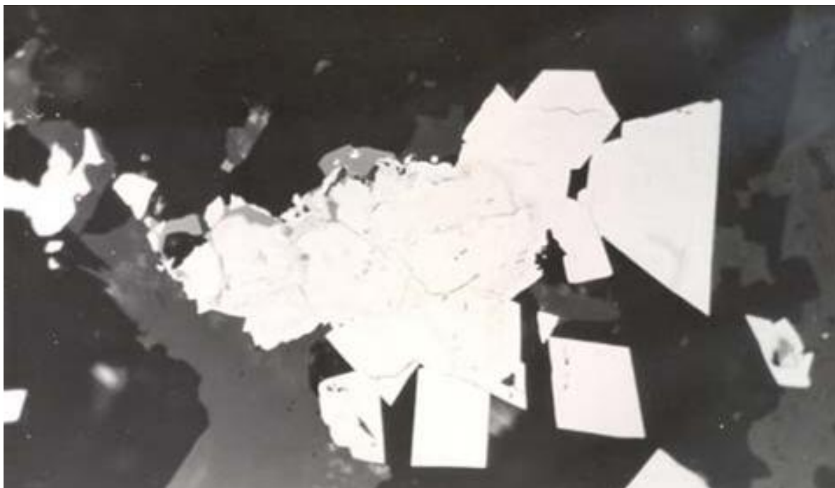
Figure 7.18: Idiomorphic crystals of arsenopyrite (white) grown around a pyrite-marcasite (greyish white), with sphalerite plaques (grey) tetrahedrite and galena. Polished section x175 (source: Ravagnani and Santambrogio, 2013).
