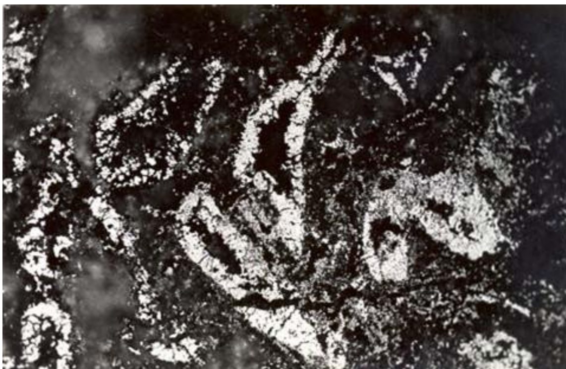
Figure 7.16: Reniform structures of pitchblende made by tiny spherulites within a carbonaceous material. Polished section x175 (source: Ravagnani and Santambrogio, 2013).
