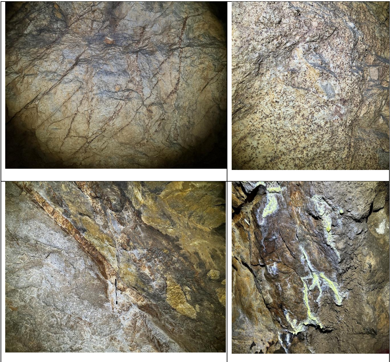
Figure 7.14: Example styles of Uraninite (Pitchblende) mineralisation at Novazza, clockwise from top left – sheeted vein/stockwork, disseminated, secondary dissolution, massive vein (source: Ravagnani and Santambrogio, 2013).
