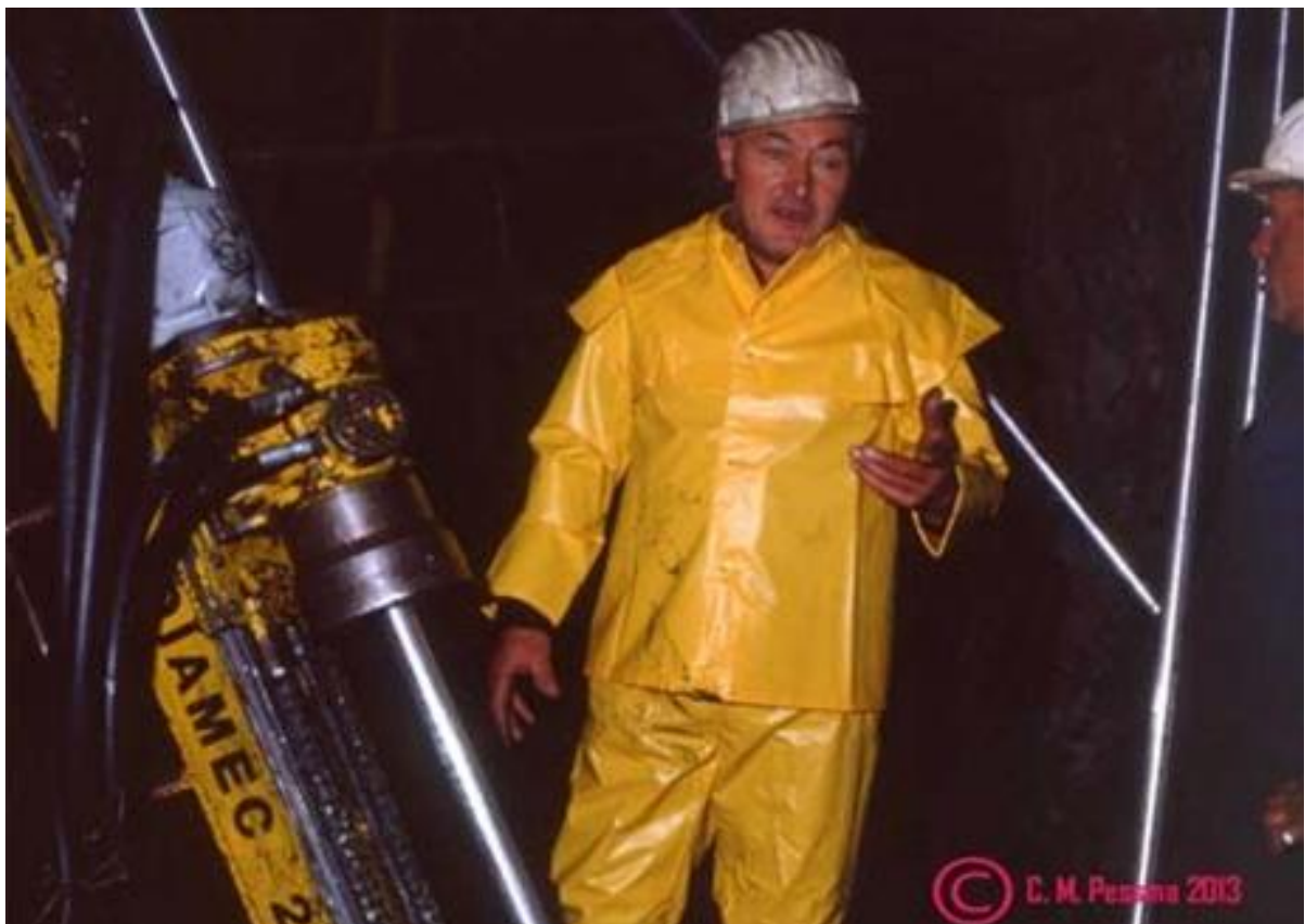
Figure 10.2: Val Vedello, Level 1 showing an Atlas Copco Diamec 250 rig in operation (source: Ravagnani and Santambrogio, 2013).
