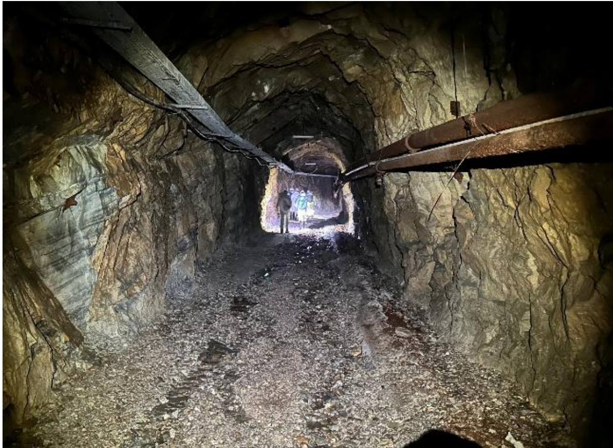
Figure 7.8: Exposure of the Novazza deposit volcano-sedimentary stratigraphy, shallow dip to SW (source: AMS, 2026).
